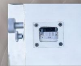
High/Low teeth indicator meter 高低齒量錶
